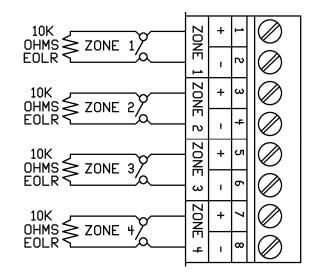
Connections to the alarm zones are as shown above. Input zones are sampled every 62mS. Changes must be present for 8 consecutive samples to pass debounce. This gives each zone a 500mS response time.
