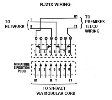
The S/FDACT is electrically isolated from the telephone lines so that a ground fault on a telephone line does not fault the S/FDACT, and the S/FDACT complies with FCC requirements.
