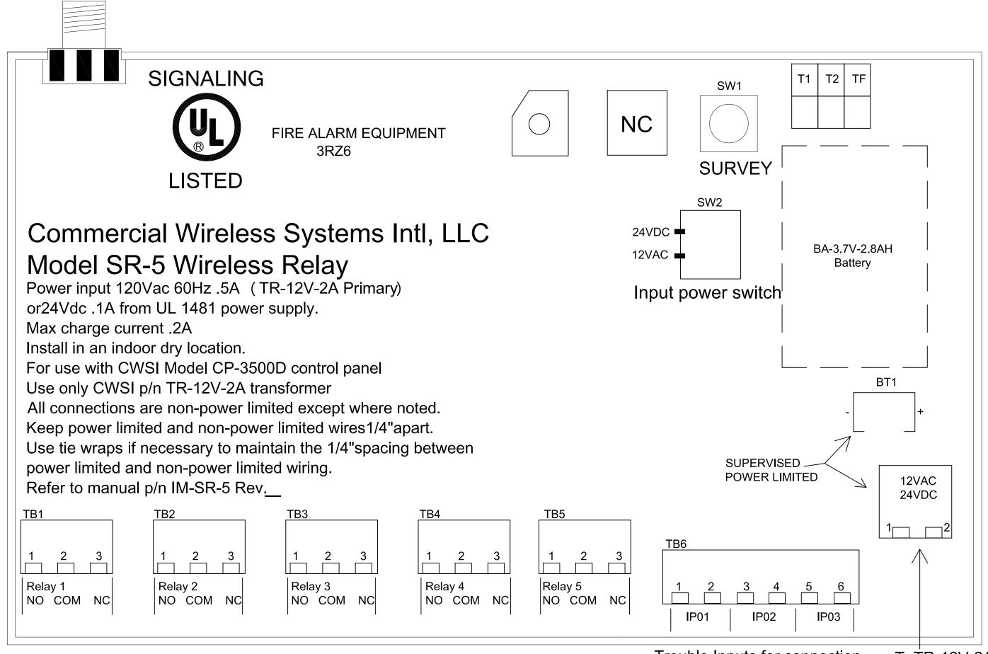
Form C outputs rated 30Vdc 5A non-power limited 30Vdc 3.25A power limited
